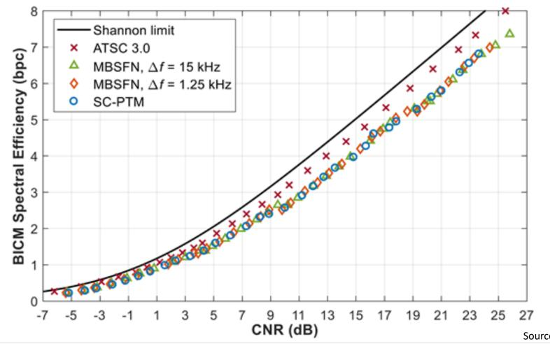
BICM Spectral Efficiency as a function of CNR for BLER=0.1% (SISO AWGN Channel)
